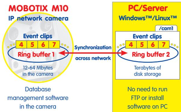
This means that in many applications central software is no longer needed to record or play back material or to scan recorded material for events. Smart network cameras provide the following functions:
