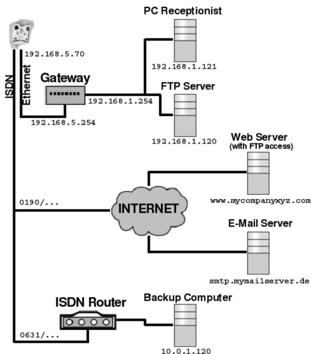
Due to security reasons, the internal company network is separated from the external network connection of the camera by a gateway. The IP addresses of the two gateway interfaces are: 192.168.5.254 (external) and 192.168.1.254 (internal). The camera is assigned the (external) IP address 192.168.5.70. The receptionist's PC has the (internal) IP address 192.168.1.121 and in the case of an alarm, the camera is supposed to store images via FTP on the Intranet server 192.168.1.120.
